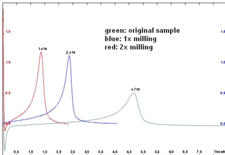
Figure 12. Monitoring conversion to hydrate in a microcalorimeter.
