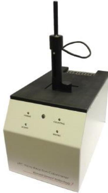
Figure 4. The THT uRC isothermal solution calorimeter
