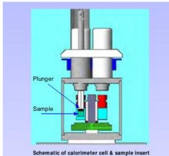
Figure 5. uRC solid/liquid mixing vessel.
