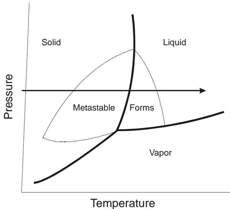
Figure 2. Example phase diagram for monotropic polymorphs.
