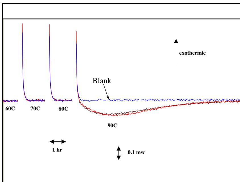
Figure 8. Monitoring isothermal polymorph conversions on a microcalorimeter.
